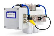
The patented Malema Interconnect Interlock Device (MIID-1000) By-Pass Leak Detection and Prevention System features all high purity PTFE and PFA construction of the wetted components and was developed especially for use in CMP tools. With built-in leak detection, monitoring, and optical valve position sensing, the MIID Interlock Device provides backflow protection and prevents internal bypass leaks in bulk chemical and high-purity water applications.
