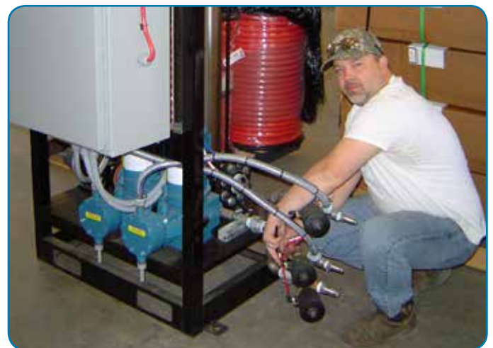
An employee at Whiting Systems checks on a pair of Neptune 7000 Series Mechanical Diaphragm Metering Pumps, which have played a prominent role in Whiting Systems’ expansion into oilfields.
