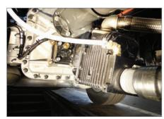
**PF Option – PTO Flange**Splined shaft for direct flange mounting on PTO
